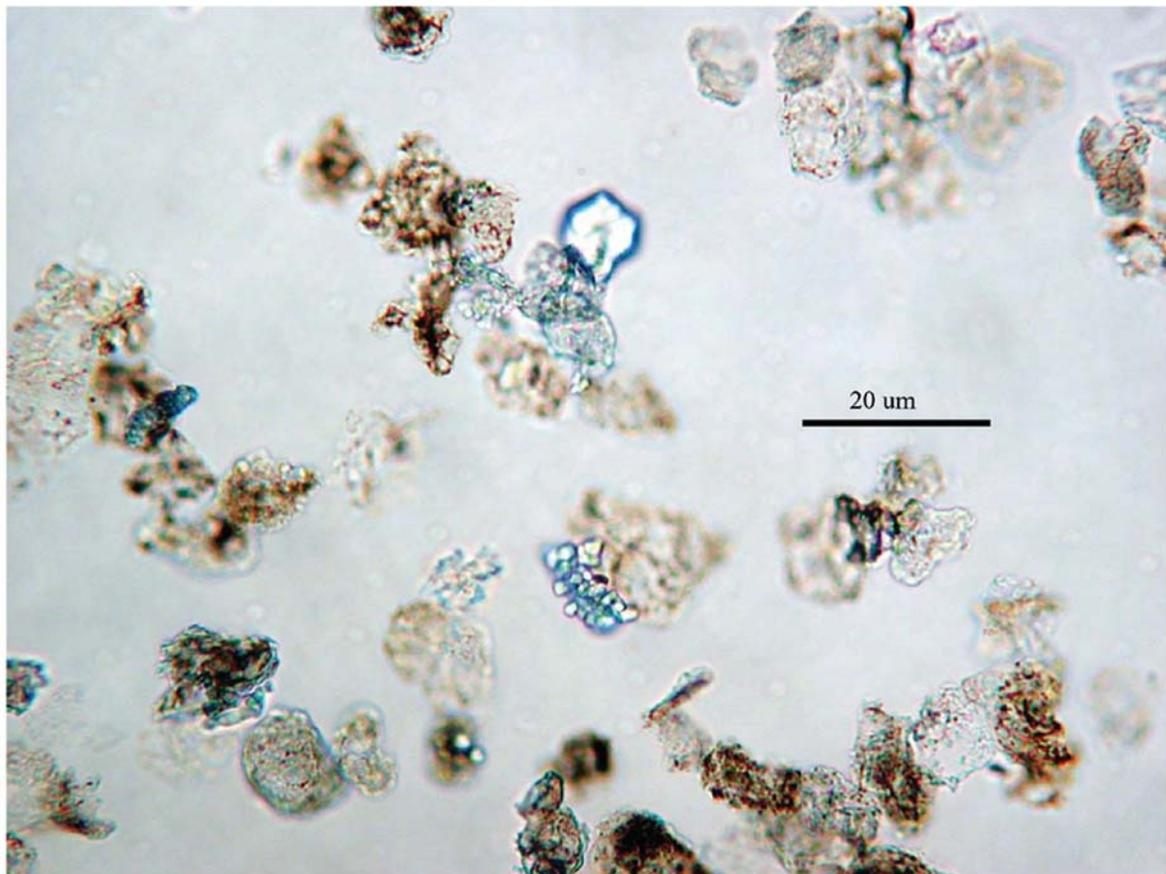
Figure 3: Polarized light microscope image of the residue obtained after backwashing a process filter used for a problem alumina slurry lot. The filter treatment details are given in the text.
