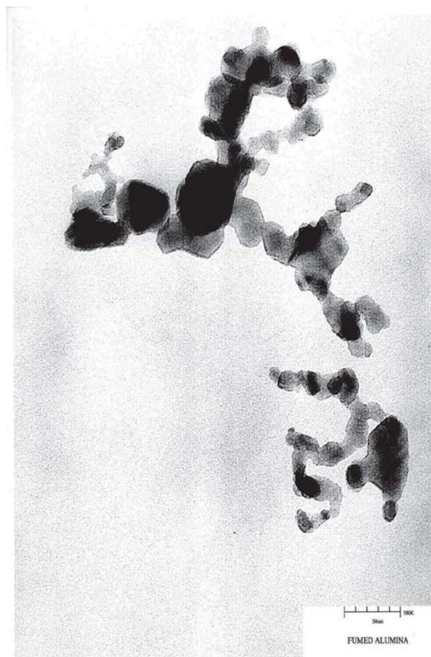
Figure 1: A transmission electron microscope image of a typical Cabot 55 m<sup>2</sup>/g fumed alumina aggregate.
