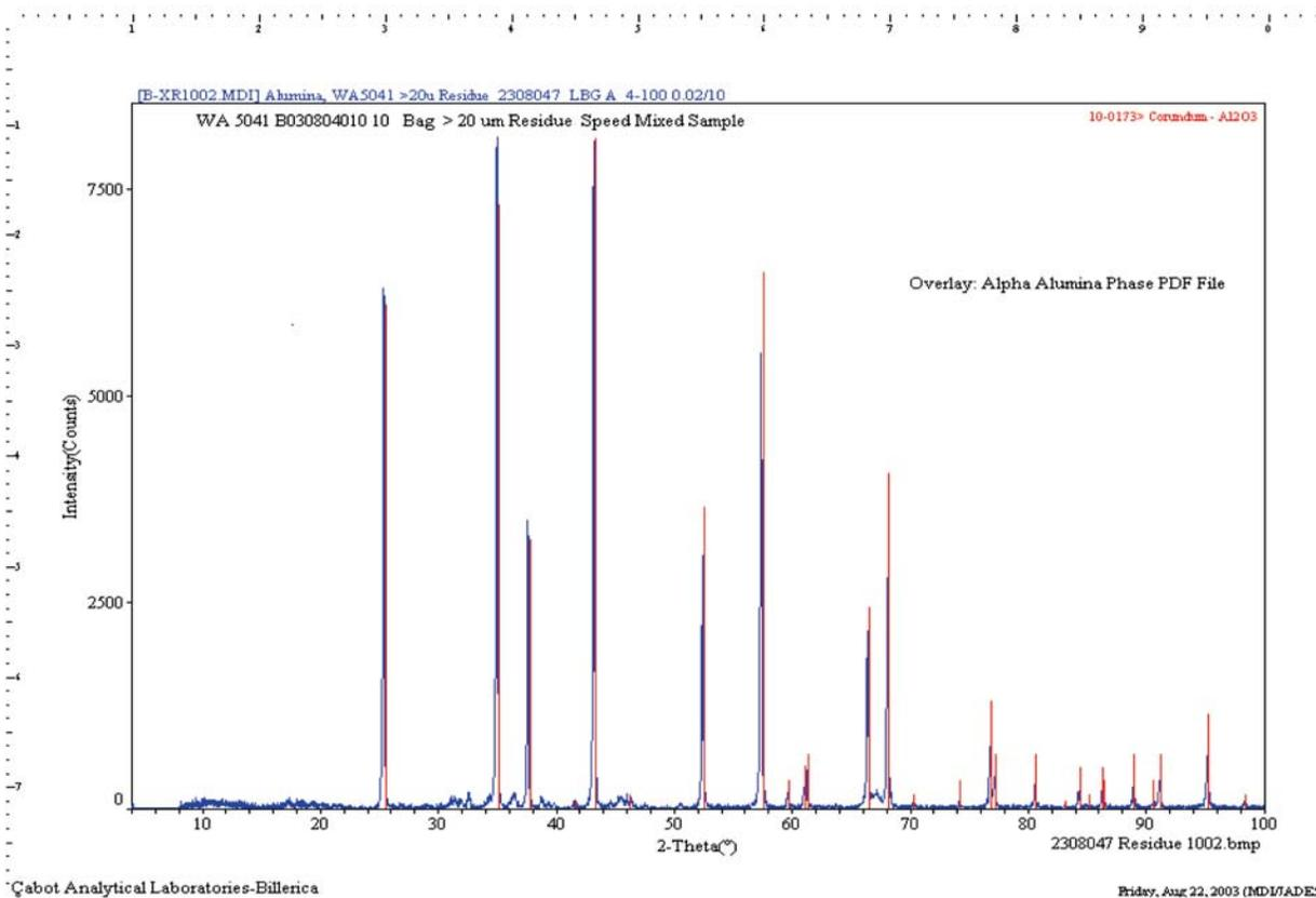
Figure 4: XRD spectrum of the same filter residue as shown in Figure 3. The red trace is the library reference spectrum of alpha alumina.
