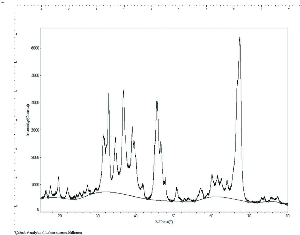
Figure 2: Powder X-ray diffraction (XRD) spectrum of Cabot 55 m<sup>2</sup>/g fumed alumina.
