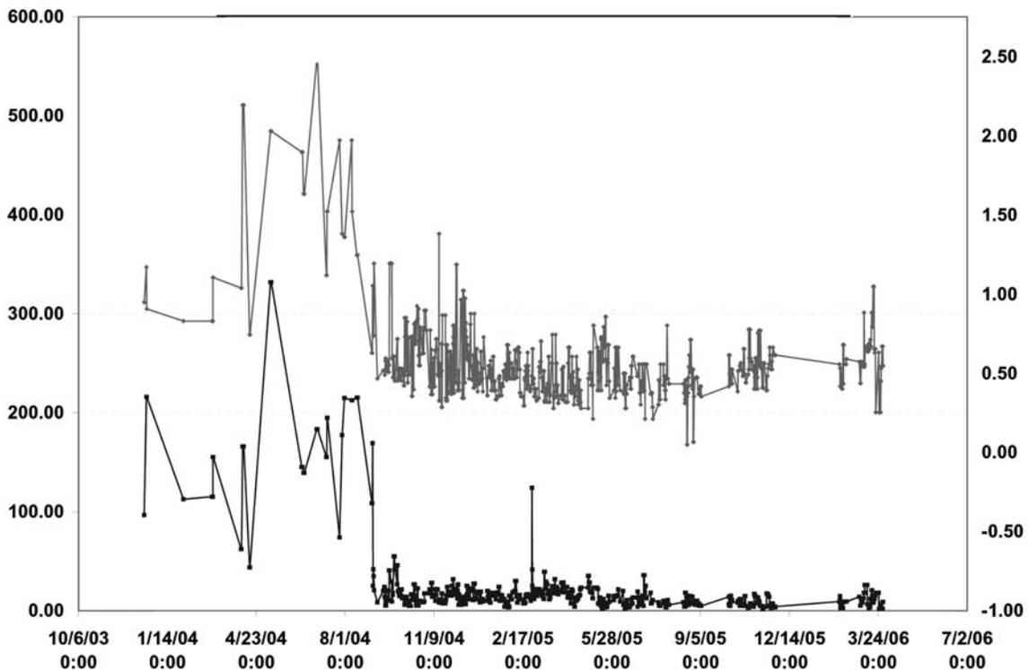
Figure 5: Results from the PLM alpha alumina count test (see text) compared with the end user filter change process data, during the problem period and after the remedial action applied to the fumed alumina production process. Comparison of user process variable (upper plot) and microscopical alpha co-count count (lower plot).
