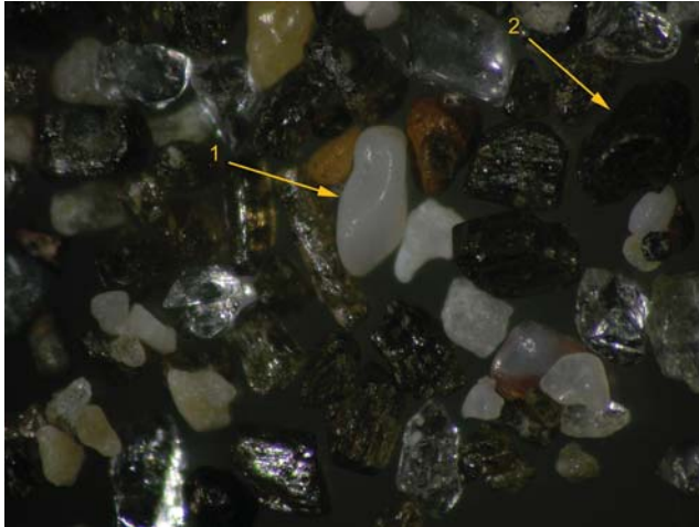
Figure 1. EV -1: Arrows denote sand grains that require different exposures to be properly imaged with reflected light.
