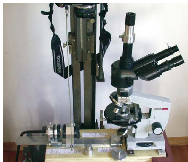
Figure 18. Photograph of the Biolam with a trinocular head and a phase telescope inserted in the right eye tube. One objective has a water immersion cap and the other objective is a 30X water immersion objective used without a cover slip. Below the trinocular head is a housing containing an analyzer and compensators in sliders. The stepped diameter bar on the wood base is used to mechanically center the aperture diaphragm with the bore of the collector lens housing.
