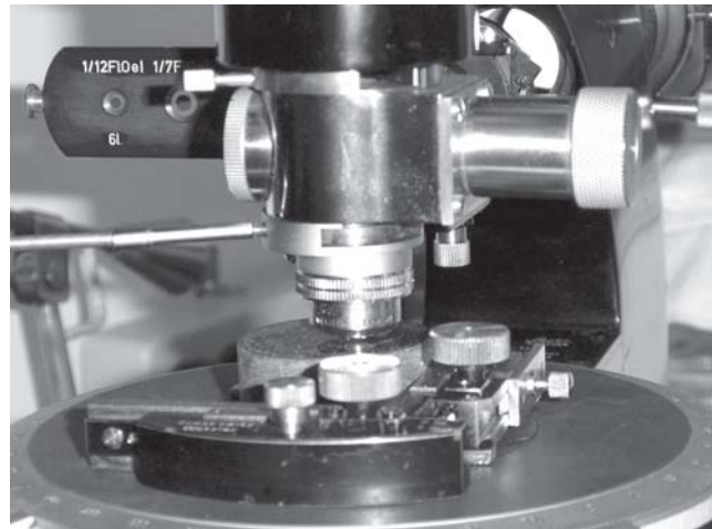
Figure 3. Photograph showing (on the left) a Stach slider of opaque stops installed in the polarized light vertical illuminator of a Leitz Ortholux microscope.
