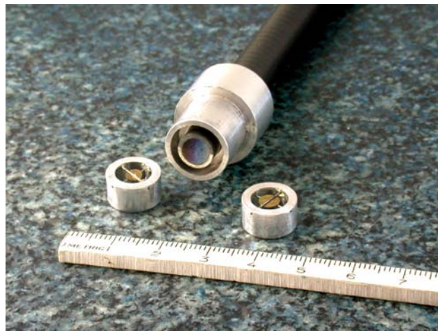
Figure 9. Close-up photograph of the ¼" light-guide end mounted in a reducing bushing with a recess for mounting the opaque stops. The stops were punched from 0.005" brass shim stock and glued onto 0.012" diameter steel wires after precise centering.
