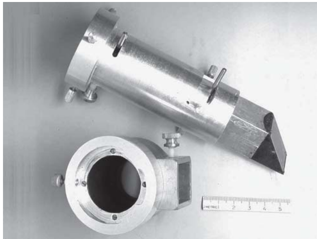
Figure 4. Photograph showing the vertical illuminator and mating housing fabricated for a Biolam microscope.
