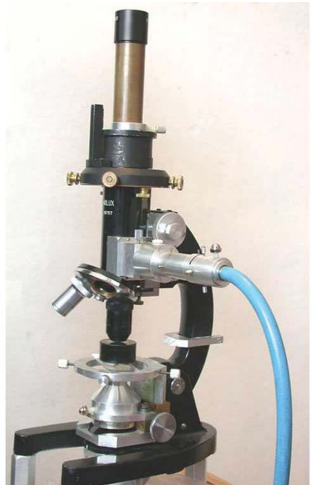
Figure 1. Photograph of the Monolux microscope equipped for reflected Köhler illumination of a metallographic specimen.
