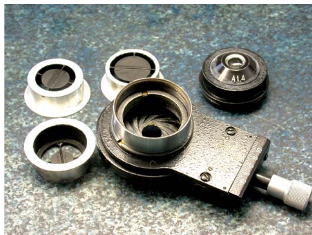
Figure 17. Photograph of the LOMO 1.40 NA aplanatic condenser with the lens housing separated to show the bore allowing the flanged stops to be inserted for either transmitted COL or darkfield.
