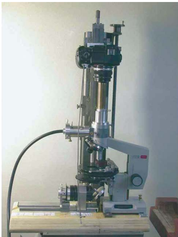
Figure 8. Photograph of Biolam set-up for photomicrography similar to Figure 7 except the shortened vertical illuminator is shown with a ¼" light-guide in place of the ½" light-guide shown in Figure 7.
