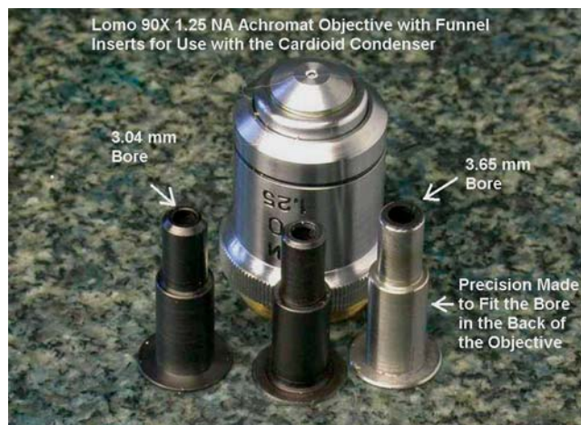
Figure 15. View of the LOMO 90X 1.25 NA objective with funnel inserts to reduce its operating NA. The precision-made funnel insert is on the right.
