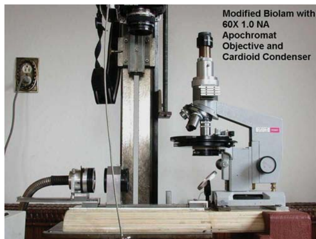
Figure 7. View of the Modified LOMO Biolam with the cardioid condenser and 60X 0.70-1.00 NA objective installed.
