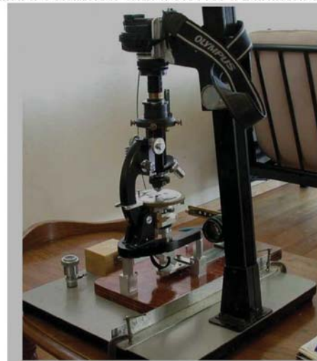
Figure 4. View of the modified Monolux system equipped with a 10X central-stop objective.
