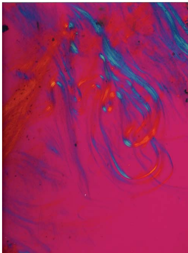
Figure 1. This image by Kristin L. Bunker shows a bundle of fibrils of chrysotile asbestos with prominent "knees." Microscope conditions include crossed polars and a Red I compensator. Replication of color in the photomicrograph compared to actual view under the microscope is excellent. Illumination in the field of view is balanced, and the natural effect of the fibers displays an ethereal artistic quality.
