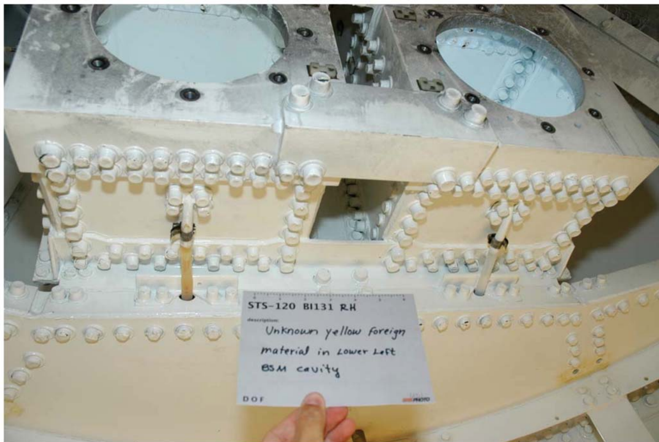
Figure 1. Yellow unknown material in frustum drain tube
