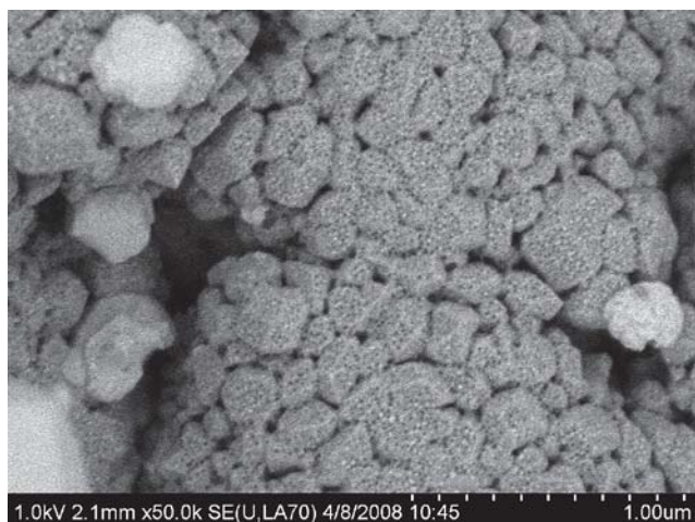
Figure 9. SEM image of AAO crystallites at 50,000X magnification.
