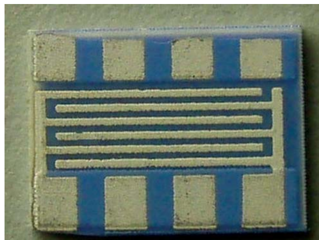
Figure 5. Planar view of finished AAO sensor. Sensor dimensions are 0.500 x 0.400 of an inch. Thin-film processing was employed to synthesize the underlying oxide layer; thick-film methods were used to pattern the electrodes and interconnects.
