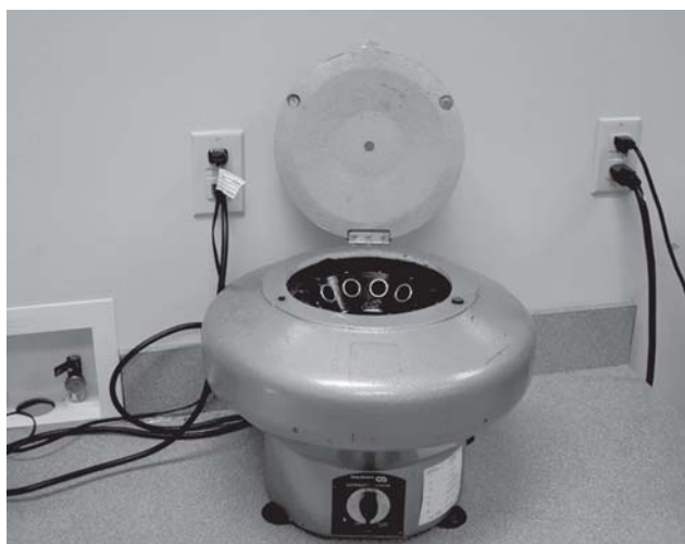
Figure 2. Centrifuge used in acid/base digestion process.
