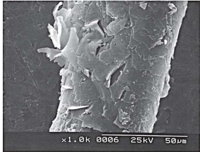
Figure 2. SEM micrograph showing disrupted cuticular scales, 1000x magnification at 25kV.
