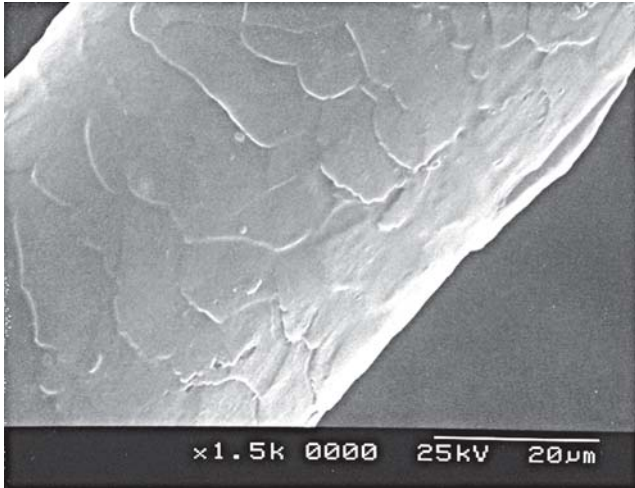
Figure 1. SEM micrograph showing intact cuticular scales, 1500x magnification at 25kV.
