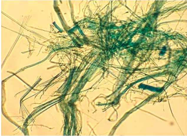
Figure 13. Malachite green stained NIST SRM 1866 chrysotile leached for 24 hours, viewed in plane polarized light at 100X magnification.
