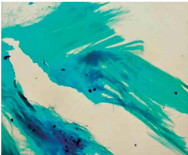
Figure 11. Malachite green stained Quincy-sur-Cher sepiolite control, viewed in plane polarized light at 100X magnification.
