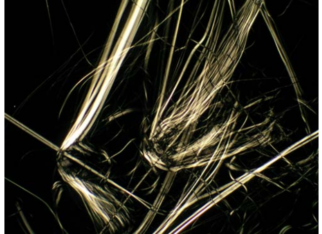
Figure 2. Theftord Mines orthochrysotile viewed in crossed polarized light at 200X magnification.
