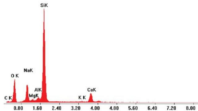
Figure 11: SEM/EDS spectrum showing a composition of primarily oxygen, sodium, magnesium, aluminum, silicon, and calcium (Sample 3).
