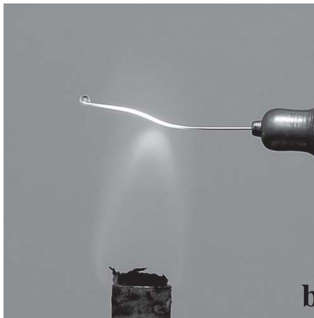
Figure 1: a) Image showing sodium carbonate/pulverized glass combination held in platinum wire loop, b) image showing the loop being heated over alcohol lamp.
