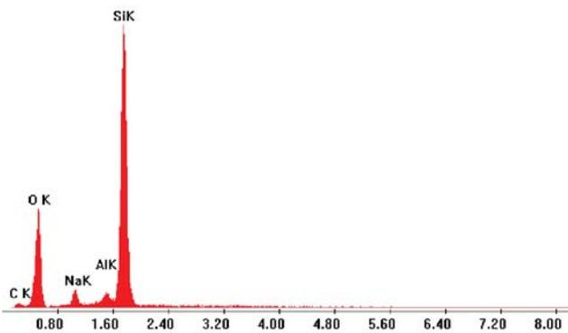
Figure 5: SEM/EDS spectrum showing a composition of primarily oxygen, sodium, aluminum, and silicon (Sample 1).
