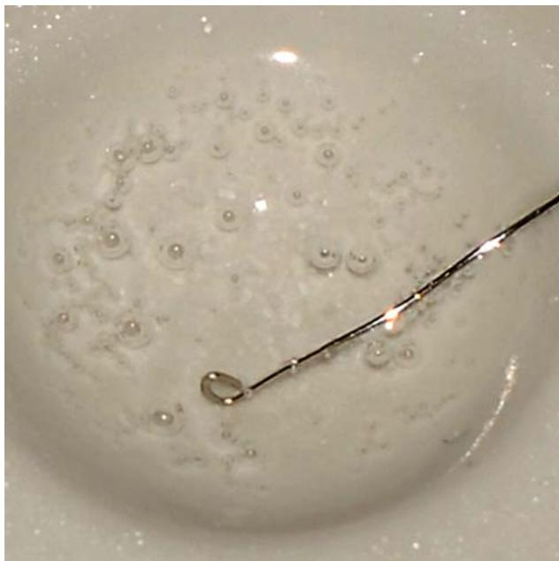
Figure 2: Image of platinum wire loop with bead of sodium carbonate and pulverized glass being submerged into 1:1 dilution of hydrochloric acid.
