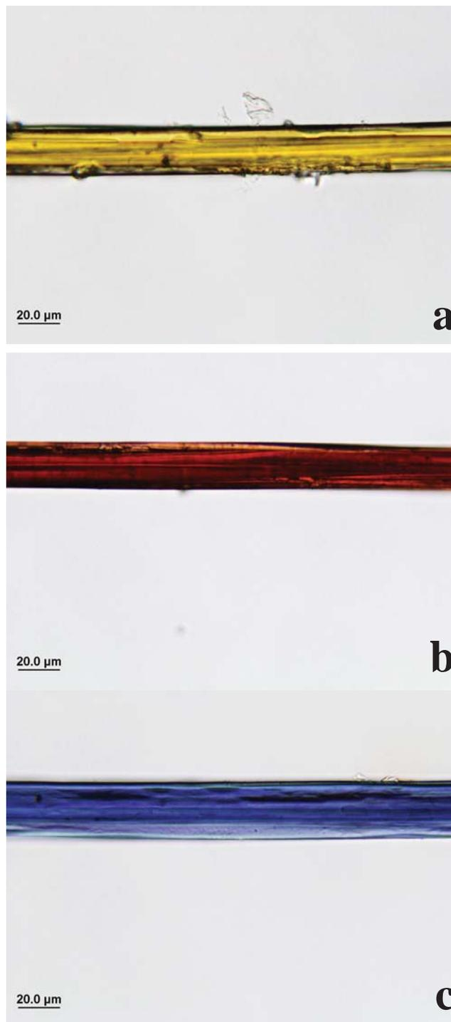
Figure 3: a) Plane polarized light image of yellow turmeric fiber, b) plane polarized light image of turmeric fiber after being submerged in test drop and showing red color, indicating possible presence of boron, plane polarized light of fiber in "b" after being treated with 1% sodium hydroxide, c) turning previously red fiber blue as confirmation of the presence of boron.
