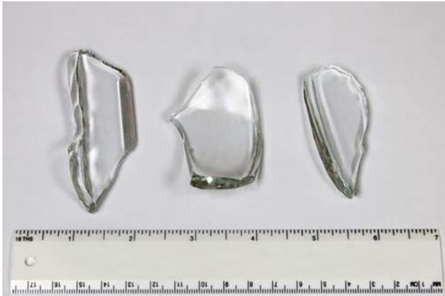
Figure 10: Broken glass fragments as received for analysis (Sample 3).
