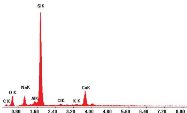
Figure 8: SEM/EDS spectrum showing a composition of primarily oxygen, sodium, aluminum, silicon, chlorine, and calcium (Sample 2).
