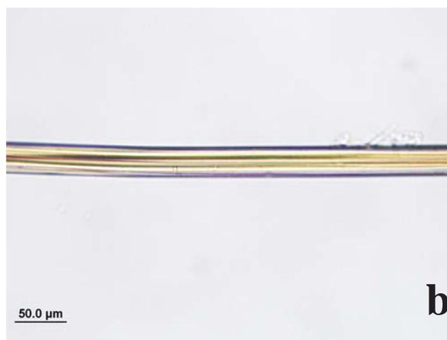
Figure 9: Chemical test for boron (Sample 2). a) Plane polarized light image of the test fiber before addition of sodium hydroxide solution, b) same test fiber after addition of sodium hydroxide solution.
