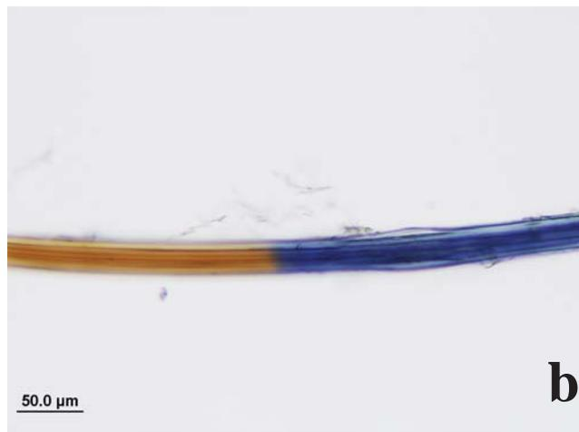
Figure 6: Chemical test for boron (Sample 1). a) Plane polarized light image of the test fiber before addition of sodium hydroxide solution, b) same test fiber after addition of sodium hydroxide solution.
