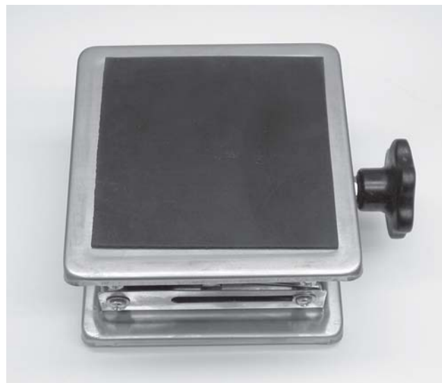
Figure 5. A laboratory jack used to raise and lower the potassium hydroxide solution.
