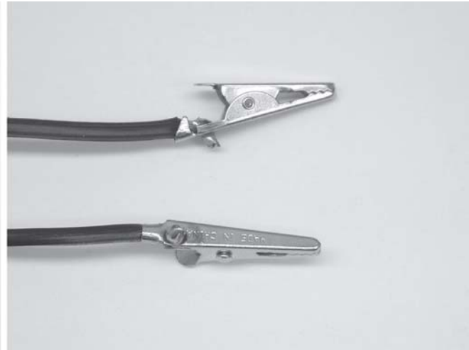
Figure 3. The cut end of the power cord shown after splitting (left) and with alligator clips soldered to the wires (right).
