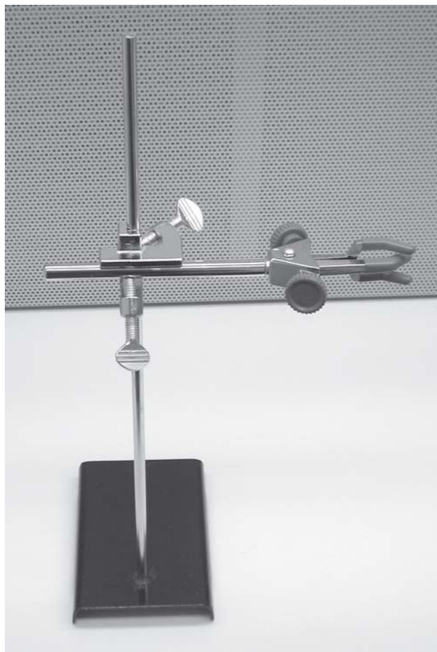
Figure 4. The support system assembled to hold the wires for tungsten needle sharpening.
