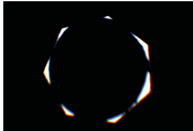
Figure 4. Back focal plane of DS objective. Condenser aperture is closed to an "eclipse" position.
