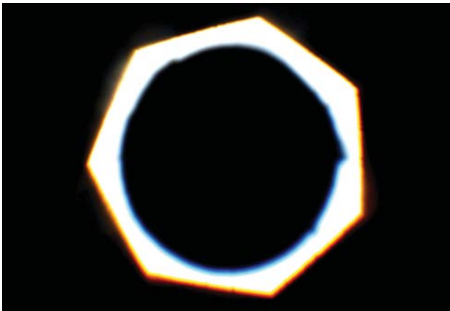
Figure 3. Back focal plane of DS objective. The central stop is centered with respect to the condenser aperture.
