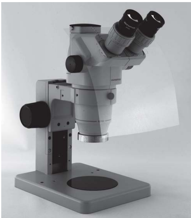
Figure 4. A finished microscope shield made from a plastic transparency.
