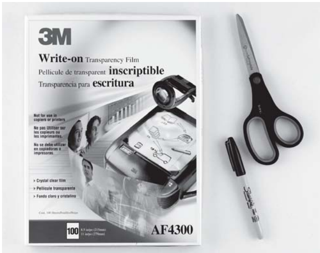
Figure 2. Transparency sheets used for overhead projector presentations are an inexpensive alternative to commercial shields and can easily be customized to fit any microscope.
