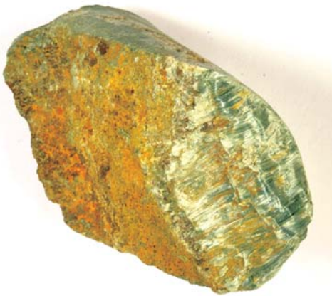
Figure 2. Rock samples used in the test program to demonstrate the effect of comminution on rocks potentially containing asbestos minerals: 2A, serpentine rock collected at the mine in Lowell, Vermont; 2B, pieces of rock containing tremolite asbestos that was obtained from a drill core; 2C, a sample that is also from a drill core but contains actinolite (byssolite); and 2D, two pieces of chrysotile ore from the Lowell mine.
