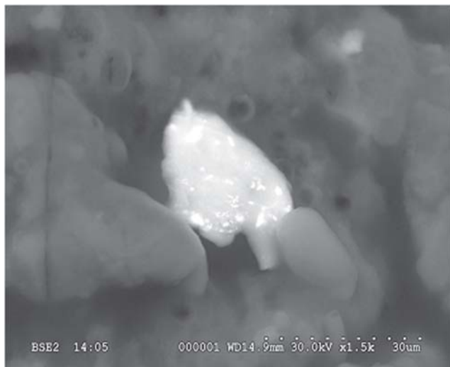
Figure 19: One of several iron-containing particles in the green stain.
