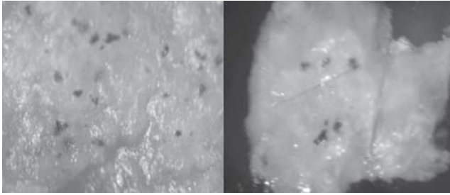
Figure 23: Left photo: Grey discoloration of cheese sauce packaged in a plastic pouch. Right photo: Grey discoloration and a white residue after the washing away the cheese sauce with water.
