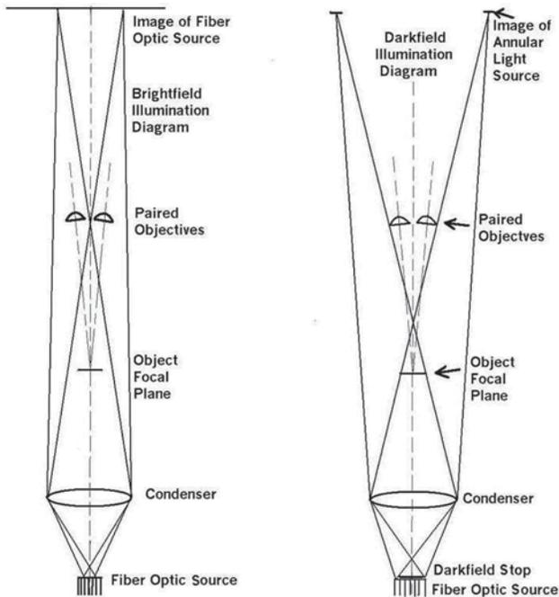
Figure 2. Schematic ray diagram for the multimode illuminator shown in Figure 1.
