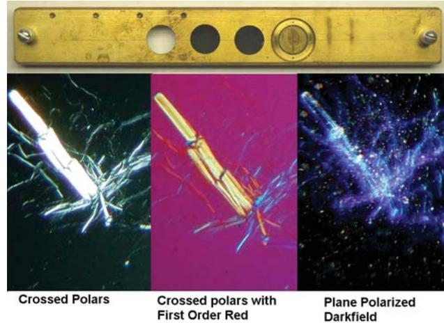
Figure 3. Top: The slider from the multimode illuminator has a clear opening for brightfield illumination and inserts in the other openings for polarized light, a first order red compensator and darkfield illumination. Bottom: Images of chrysotile asbestos in 1.550 mountant taken with the slider.
