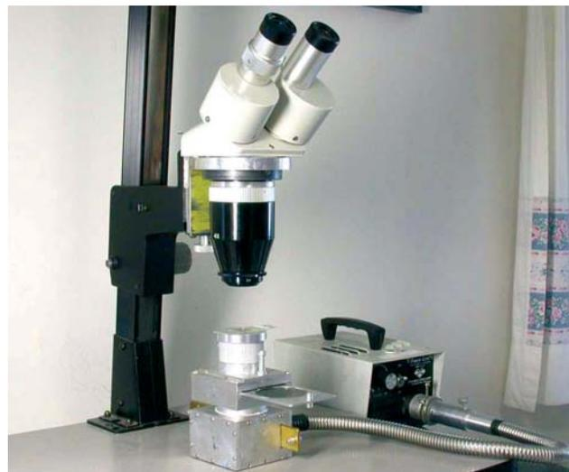
Figure 1. Meiji stereomicroscope with the home-built multimode transmitted light illuminator.
