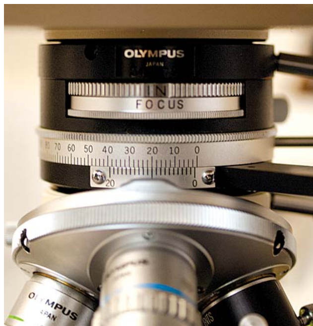
Figure 11. An Olympus Bertrand lens location (focusable) at the "IN" position above the analyzer (graduated) and Red I waveplate. Below the analyzer and waveplate is the turret for the objectives.
