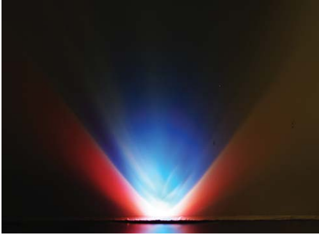
Figure 14. An X-sectional display of a Rheinberg cone of light with a two-color set-up (inner center of blue and outer ring of red), using Robert E. Smith's technique (see References Cited, No. 72). Note that the inner cone has a higher intensity (more brightness).
