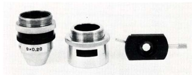
Figure 5. A 9X objective with built-in iris (left) is standard for the MPD-1. A slotted "extension" tube for the objective takes a slider as shown center and right.
