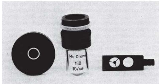
Figure 4. Dispersion staining objective with central-stop slider removed; on the left is a substage condenser annulus for use with a 40X phase objective.
