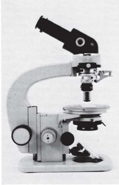
Figure 1. Side view of the Russian-made MPD-1 portable polarizing microscope, with dispersion-staining objective.
