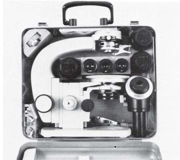
Figure 6. MLD-1 microscope in metal carrying case.
