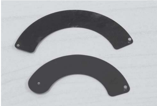
Figure 5. Upper leaf is from the Nikon Optiphot-POL, note the leaf is symmetrical. Lower leaf is from a Nikon Alphaphot. Note that one end is curved meaning that there is only one orientation in which the leaf will fit into the FD.
