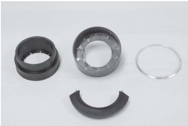
Figure 13. Individual FD components ready for re-assembly.
